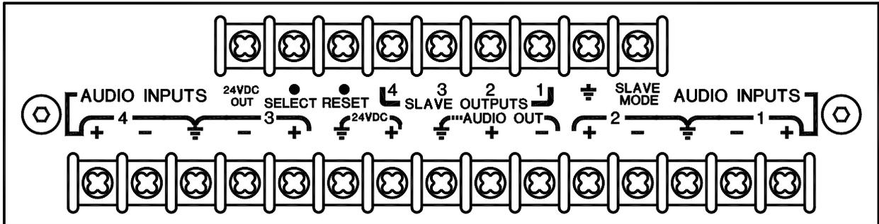
**AUDIO INPUTS:** Four audio inputs are provided. Each input may be wired balanced or unbalanced. For balanced operation, connect the input cable shield to ground, and connect the balanced leads to + and -. For unbalanced operation, connect the input cable shield to ground, connect a jumper from ground to the - input, and connect the unbalanced signal lead to the + input terminal.
