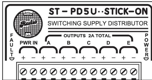
24 Vdc power is distributed to up to 5 modules. It is not necessary to use all 5 outputs. The red **POWERED** led is illuminated when the initial powering ramp cycle is complete and the outputs are being supplied directly by the power supply. Ground referenced and SupplyFlex modules may be powered from a common ST-PD5U power distributor.
