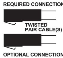
Connection from Single-Pair, Two-Pair or Three-Pair Senders (direct, or via an RDL Twisted Pair Power Inserter)
