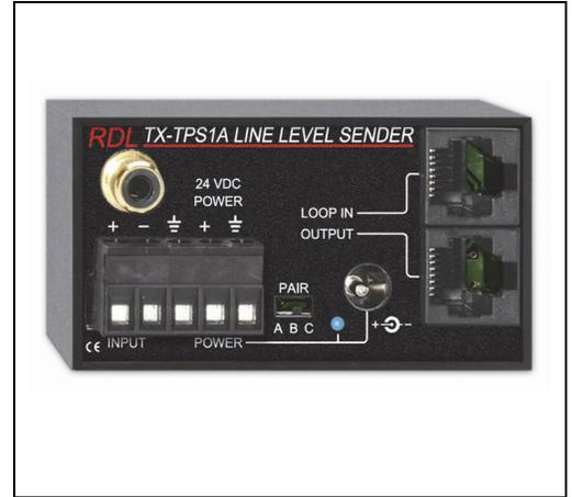
The TX-TPS1A is a single-pair audio sending module compatible with RDL Format-A twisted pair products. It is built in the versatile Max-TX series enclosure. The durable adhesives provided with the TX-TPS1A permit permanent or removable mounting. The TX-TPS1A may be rack or surface mounted with optional TX™ series accessories.
