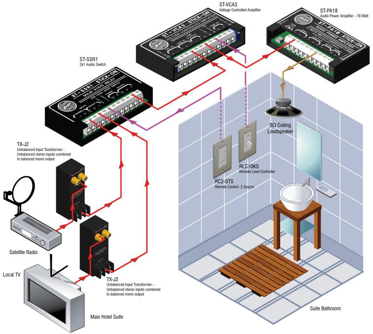
The compact size of RDL modules allows the creation of a system to provide high quality sound in a nearby room without dedicating space for electronic equipment. The example pictured allows remote level control and source selection using equipment which can be placed in electrical boxes or tucked into a TV armoire.
