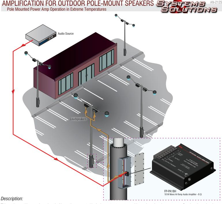
This outdoor parking area is equipped with speakers mounted in the lamp structures to provide music and paging coverage. Speakers in each pole are powered by an RDL FP-PA18H 18 Watt Hi-Temp Audio Amplifier. The amplifier module is mounted in an unventilated watertight enclosure at the base of each pole. The poles recieve direct sunlight causing the potential for high internal ambient air temperatures.
