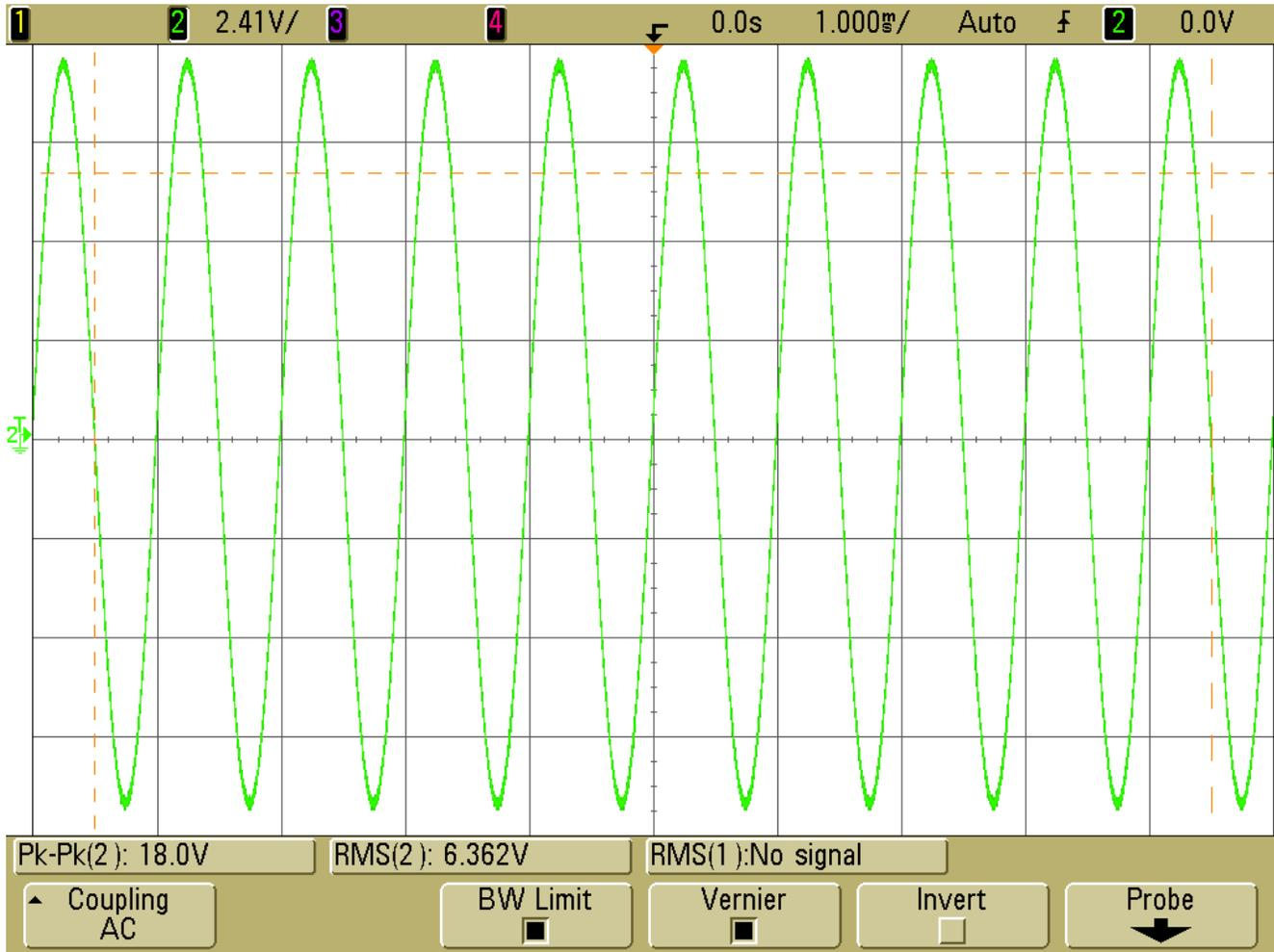
Prior to applying the speech source, the amplifier was first fed with a sine wave. The vertical input sensitivity was set to maximize the waveform on the screen. Peak-to-peak and RMS automatic measurements were selected and the cursor was enabled to indicate the amplitude of the calculated RMS voltage. The applied tone produced the following reference readings to be used in subsequent speech audio tests:
