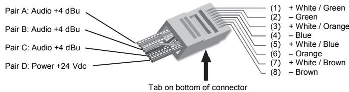
RJ45 conductor colors shown are for 568A standard. The 568B standard may be used if the connectors at both ends of the cable are wired identically.
