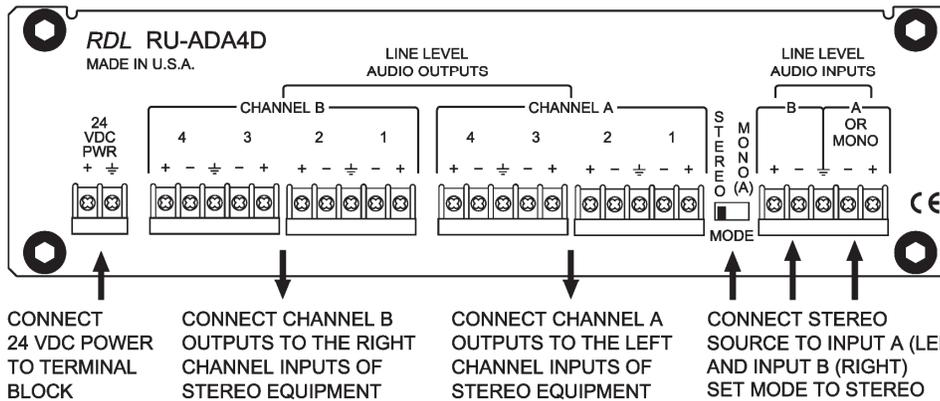
NOTE: IF THE MODE SWITCH IS SET TO MONO, THE MONO SOURCE WILL FEED ALL OUTPUTS.
