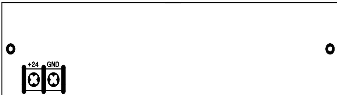
**POWER CONNECTION:** Connect a single-ended 24 Vdc power source to the **+24** terminal. Connect the ground return from that supply to the adjacent **GND** terminal. Power supply and circuit grounds are common.
