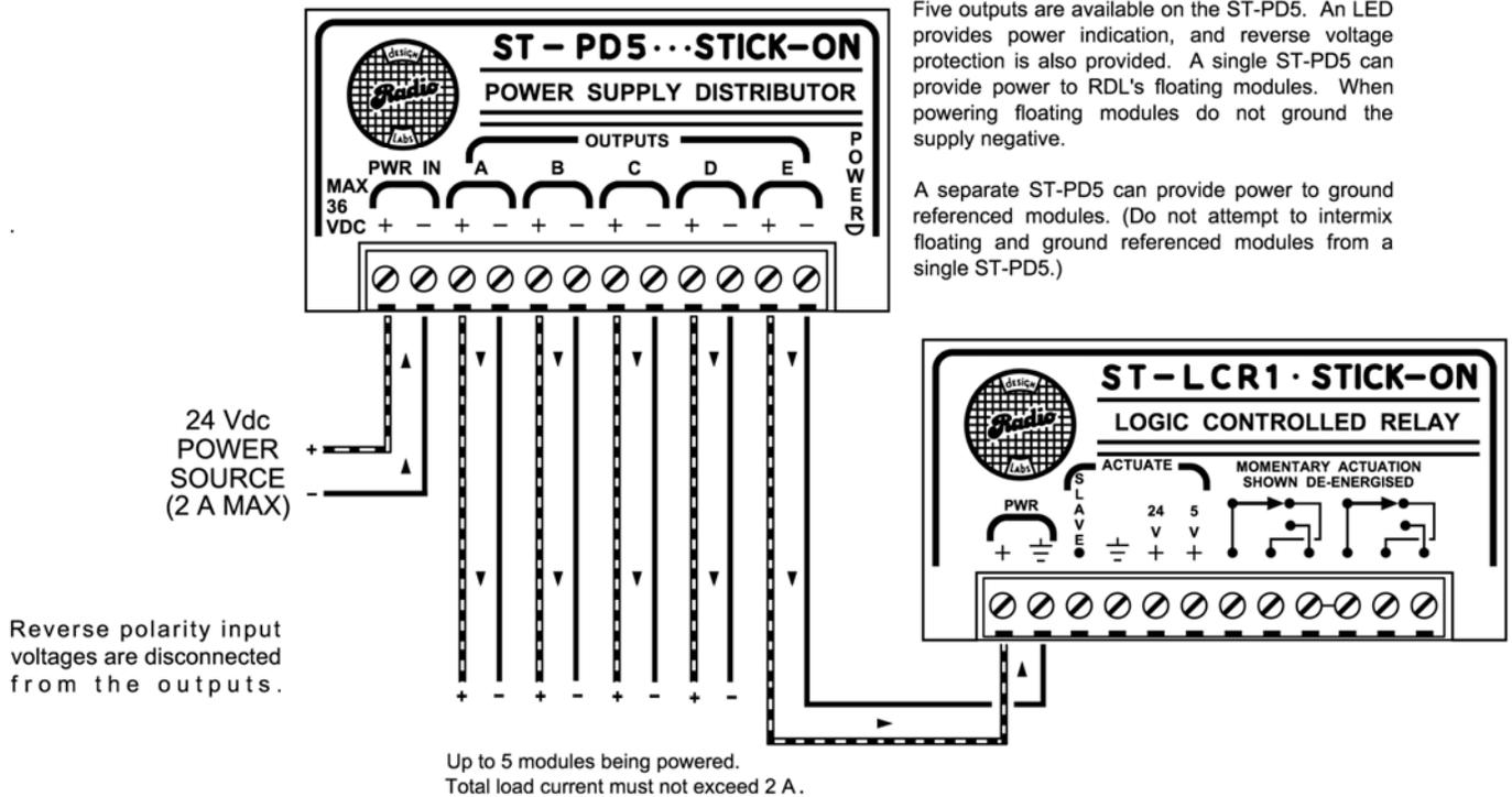
**Mount ST-PD5 adjacent to the modules it feeds (wiring not to exceed 1m).**
