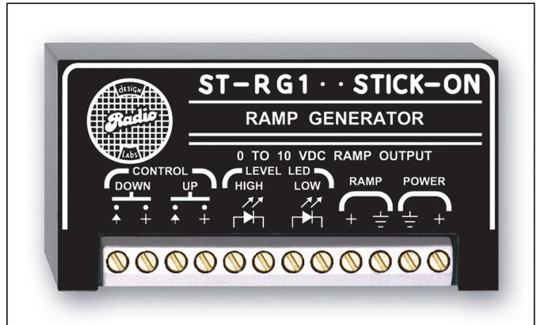
The ST-RG1 is a digitally generated 0 to 10 volt Ramp Generator in the group of STICK-ON series products by Radio Design Labs. These products are designed for quick, convenient installation and reliable operation in a variety of control applications. STICK-ONS are designed, built and rated for continuous duty in professional A/V systems.
