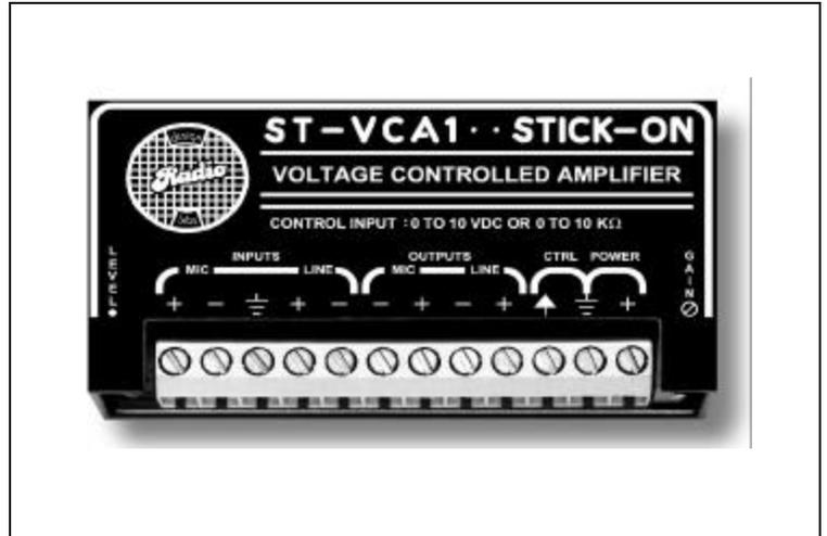
The ST-VCA1 is a high-quality Voltage Controlled Amplifier (VCA) in the STICK-ON series of products from Radio Design Labs. This VCA is designed to give you the maximum flexibility in application. Audio inputs and outputs are provided for both microphone and line-level signals. So the VCA can be used as a remote-gain-controlled mic preamp with line-level output, or can even control a line-level signal feeding into the mic channel of a mixer.
