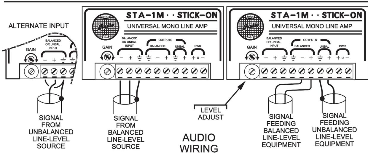
IT IS USUAL TO NOT CONNECT BALANCED OUTPUT SHIELD TO REDUCE GROUND LOOPS
