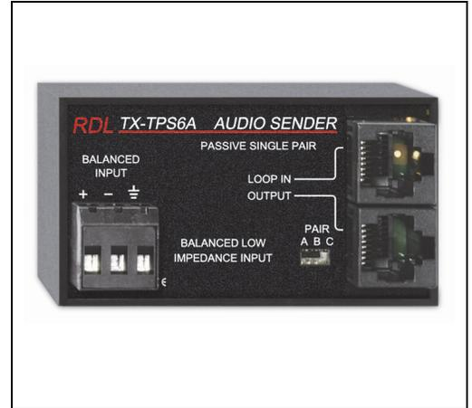
The TX-TPS6A is a single-pair audio sending module compatible with RDL Format-A twisted pair products. It is built in the versatile Max-TX series enclosure. The durable adhesives provided with the TX-TPS6A permit permanent or removable mounting. The TX-TPS6A may be rack or surface mounted with optional TX™ series accessories.
