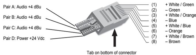
RJ45 conductor colors shown are for 568A standard. The 568B standard may be used if the connectors at both ends of the cable are wired identically.
