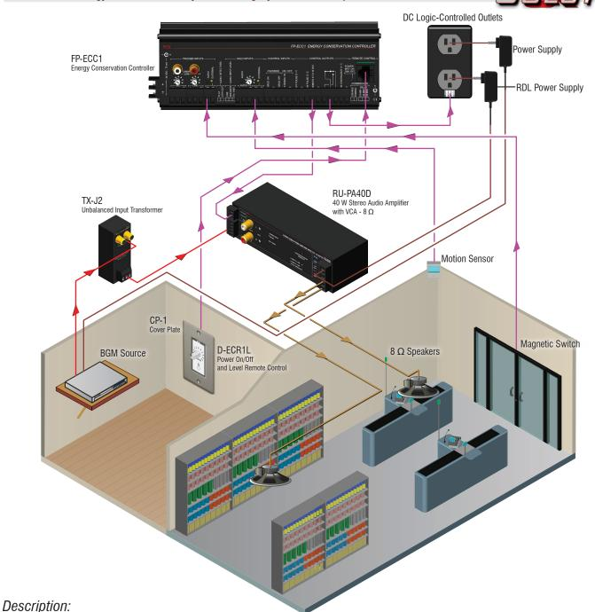
To conserve energy and reduce operating costs, the RDL FP-ECC1 Energy Conservation Controller is used to automatically power up the background music system in this retail store when needed and to power down the equipment when not needed.
