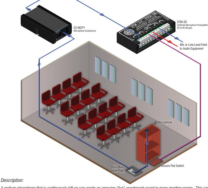
A podium microphone that is continuously left on can create an annoying "live" reverberant sound in many meeting rooms. This can be distracting before and after meetings and during breaks. This application shuts the microphone off when no one is at the podium. keeping the public address system guiet when no one is speaking.
